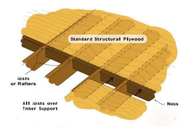
Typical ITI TImspec Structural Plywood
