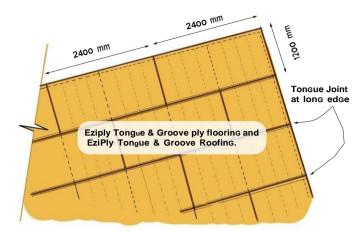
Maximum Spacing @ 400 mm Fixings @ maxiumum 150 mm to all edges and 300 mm to Central Joists
