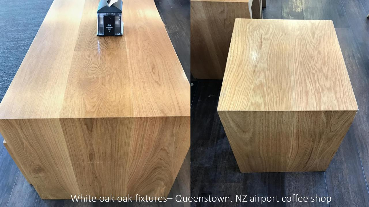
White oak possesses a cell structure called "tyloses" that closes the pores, making it resistant to water and rot. One way to tell the difference between red and white oak is to look at the end grain. If you can see tiny pin holes in the pores, it is most likely red oak.
